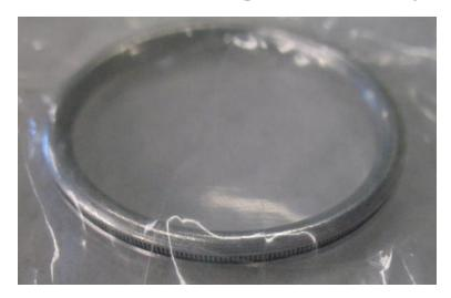
Aluminum Helicoflex c-seal with internal inconel spring. Surface finish of flange is about 80 micro-inch (2 microns). Seal is designed specifically for this finish.
